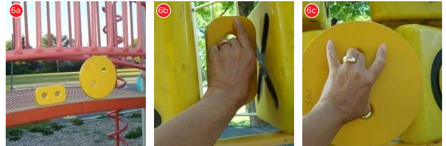
This photo shows the use of entrapment templates as opposed to the three dimensional probes.
