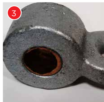
This bushing (red) is worn and should be replaced.
